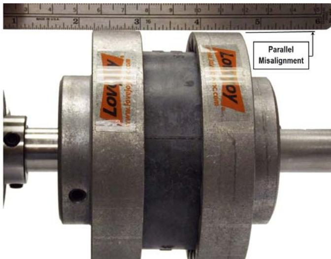
**6.12 Using a calibrated torque wrench tighten the set screws** on the second flange to the torque value specified in Table-2.
